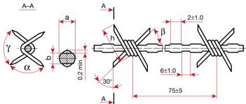
Note: angles  $\alpha$ ,  $\beta$  and  $\gamma$  – not less than 30° dimension a not less than 2.8 mm b not less than 2.3 mm h not less than 17 mm
